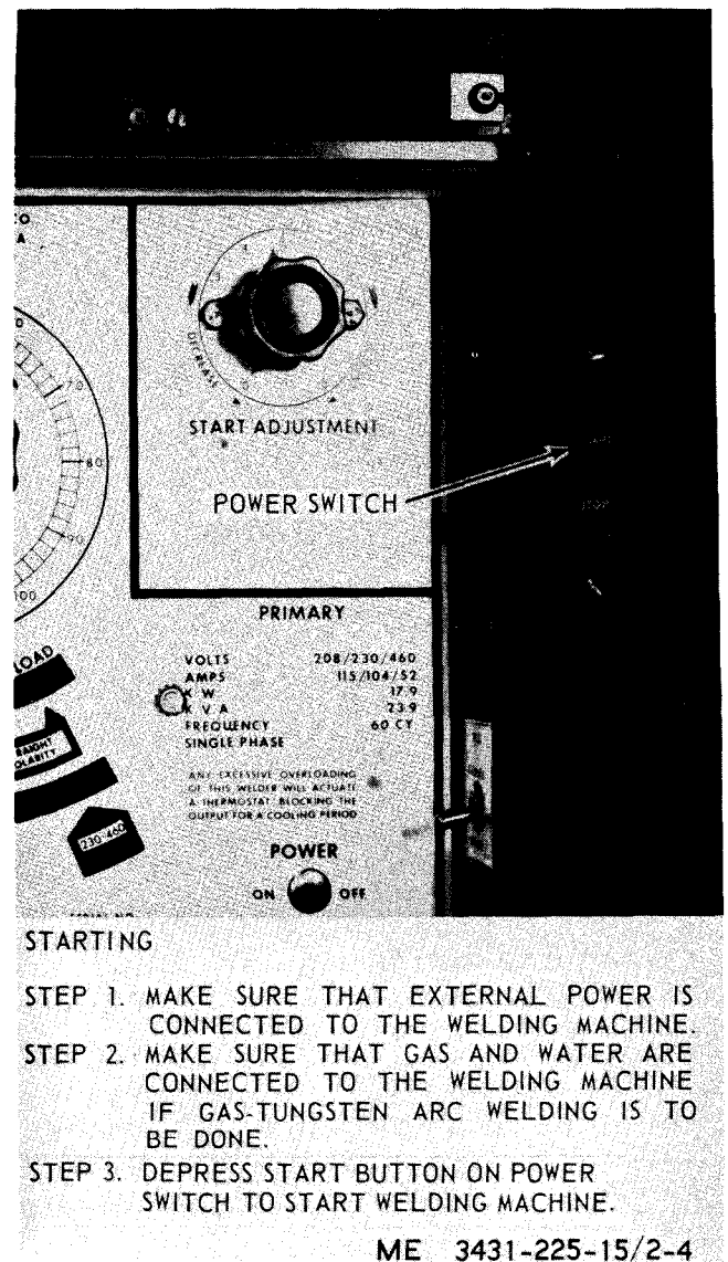
Figure 2-4. Starting the welding machine.
