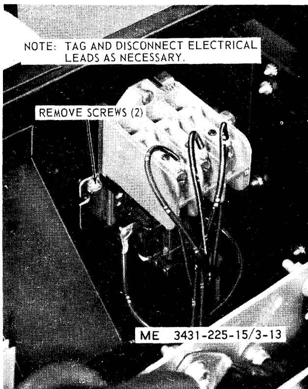
Figure 3-13. Relay contactor, removal and installation.
